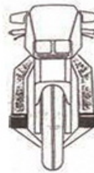
Illustration 7. Model security motorcycle equipped with side guard (metal bumper) to protect the lower limbs [ 6 ]
