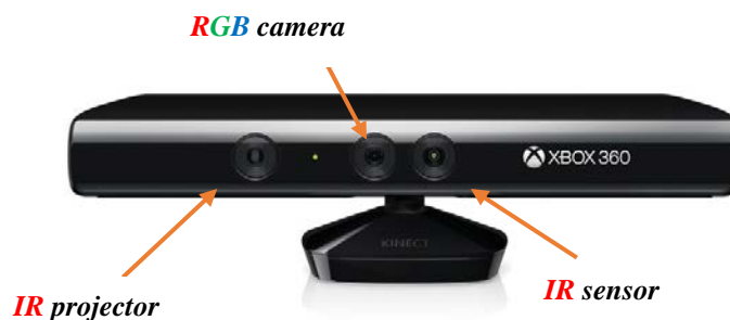
Figure 1. Locations of IR projector, sensor and RGB camera on XBOX Kinect
