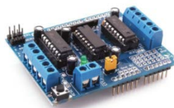
Figure 6. Module for motor control
