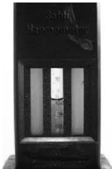
Figure 1. Hb comparator box with brown glass on either side and tube with acid hematin solution in centre. The color of the solution is matched with the glass and the concentration of Hb is read directly
